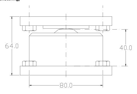
The height of 64 mm includes the isolation mount above and below the load cell.
