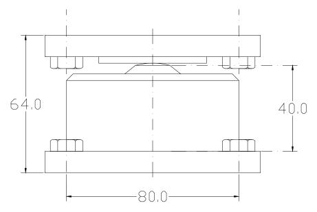
NB: The height of 64 mm includes the isolation mount above and below the load cell.
