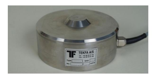
TEKFA's RBMC stainless steel compression load cell is a compact and simple load cell for applications where a load cell with high capacities is required. The applications of RBMC load cells are big-ger silo and tank plants within the food industry, chemical industry, and other demanding indus-trial environments. The load cell is produced in stainless steel with a tightness of IP68, protecting the electronics against dust and water. The RBMC series includes the capacities 20, 30 and 50 tons.
