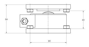
The isolation mounts over and under the load cell are inclusive of the 64 mm in height.
